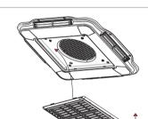
Install the air filter as shown:
