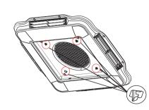
· Attach the plenum assembly to the plenum mounting bracket by engaging the two parts. You will hear four clicks to as the parts connect
