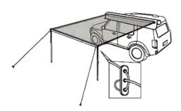
2. Open the protective cover and slide the M8\*25 bolts into the mounting rails of the tent.
