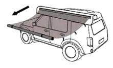
6.Use Velcro to fix the tarp to the extension pole. Use wind rope and ground nails to fix on the ground to prevent wind-blowing.
